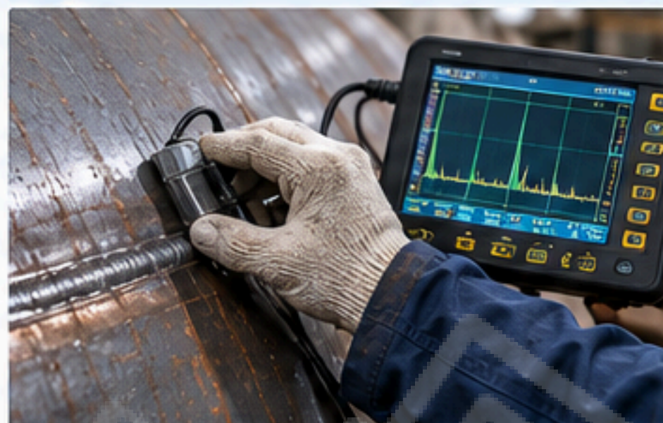
Detect internal defects such as lack of fusion, slag inclusions and cracks.
