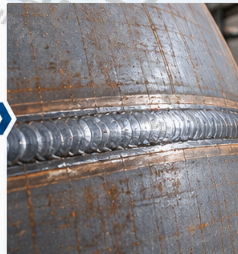
Completed Weld Seam
