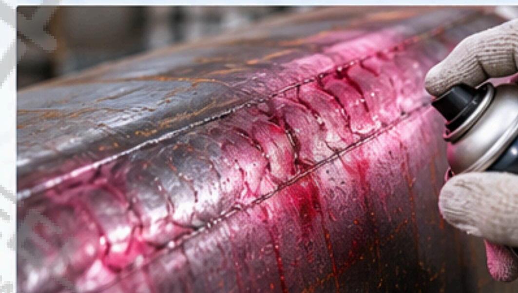
Identify surface and near-surface defects on welds.
