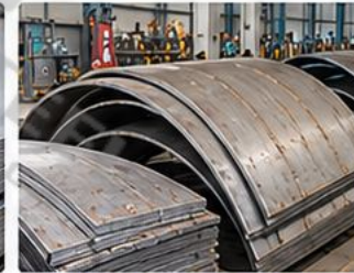
Formed Spherical Shell Plates Check material heat number and surface quality
