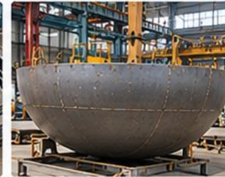
Spherical Shell Segment Dimensional and curvature inspection
